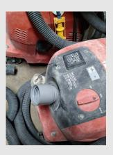
Eliminate Proprietary Connectors & *Increase* CFM: The inlet port opening on vacuums is over 2" but 1-1/4" & 1-1/2" hoses are supplied which *restricts airflow (CFM)* & *causes clogs*. Our universal cuff (D2020S) fits securely & uses 2" hose.
