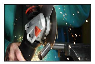
CUTS: Angle Iron, Iron Bar & Tubing, Hard & Mild Steel Ductile Iron, Rail Track, Stainless Steel, Bolts, Welds
