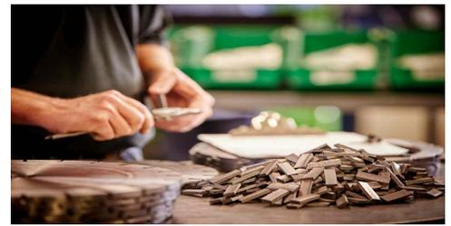
F. Diamond segments are then attached to the blade cores using the most advanced and the most strongest attachment method in the industry which is laser welding. DDM's state of the art laser-welding process uses a laser beam to fuse the segment directly to the steel core. The laser weld actually becomes as strong as the core itself. DDM's laser welding process is the most advanced in the industry.
