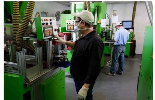
B. The manufacturing process starts with diamond segments. The metal powder and diamond crystals are precisely selected, weighted and mixed into batches. The combination of different metals and diamonds make up the bond which is specific to the geographic area of the material to be cut and the type of equipment being used.
