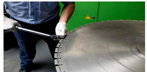
H. Blade tensioning is one of the most interesting steps in the entire manufacturing process:
