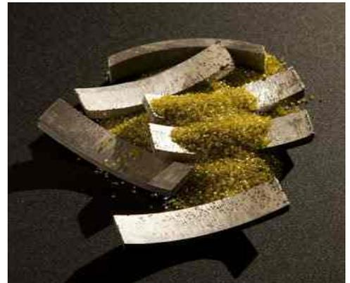
C. The metal powders and diamond crystals are measured, mixed (for hours), pressed into individual segments and weighted again on calibrated scales with accuracy to thousandths of a gram.
