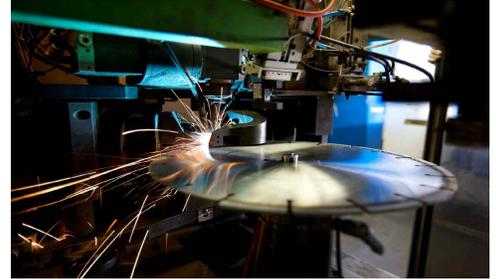
G. After the laser-welding process EVERY DDM-CONCUT blade is tested to ensure that the segments are solidly attached to the core using a torque wrench. As you can see by the photo, the segment is tested for snapping or shear strength from the steel core which, for all practical purposes, far exceeds the applicable use of any type of diamond.
