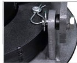
Carriage mounts with lock pins for easy removal.
